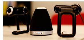
Figure 2: Capture devices, the webcam and the Microcone, used in the ELEA recordings.
